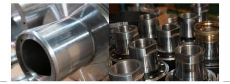
We are fully capable of grinding and polishing after plating to return parts to their size within specified tolerances.
